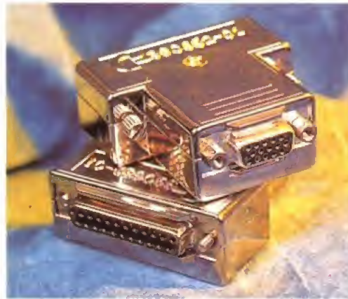
This CBM converter lets you plug a 15-pin SVGA monitor into the 23-pin video connector common to all Amigas.
